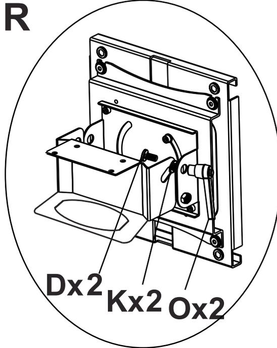
If the handle can NOT move with a full circle when TV is installed, you can press the handle, then the handle can go both clockwise and anticlockwise directions without losing the tilting mechanism.
